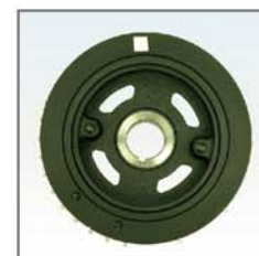
Crank pulley with Reflection Tape attached Pulse number 1
